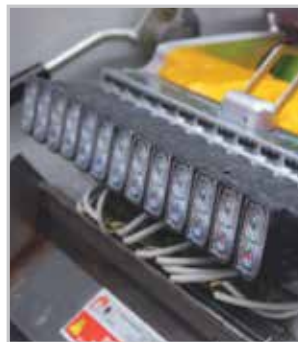
Ink fountain blade consisting of independent, fully MOTORIZED sectors
